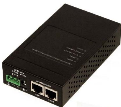
MS655400 Device Server Industriel, RS-232/422/485 vers 10/100Base-TX
